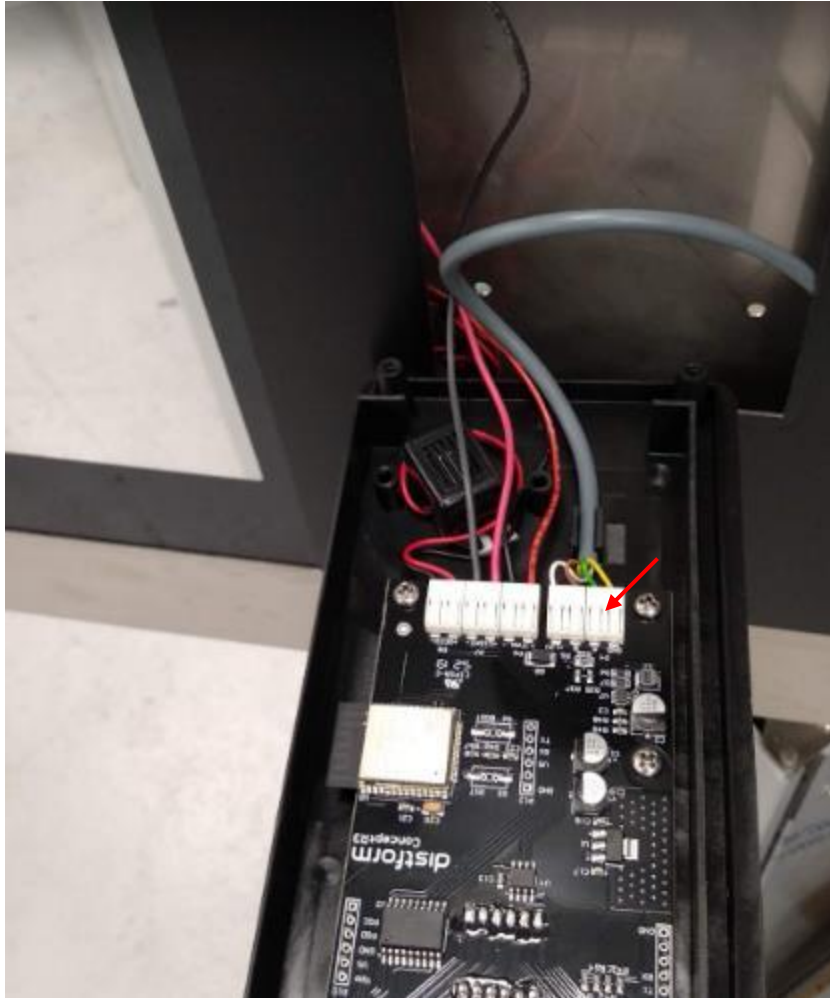
Figure 52. Release connectors. (COOK, BAKE, BAKERSHOP and SNACK) (See wiring diagram Figure 73 )
