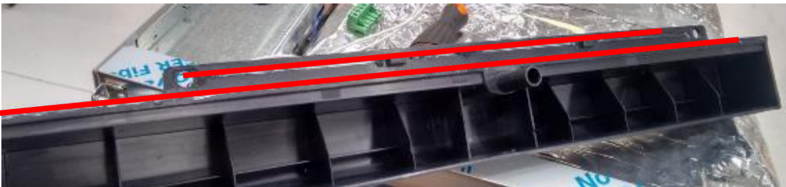
Figure 74. Silicone application on the drip tray
