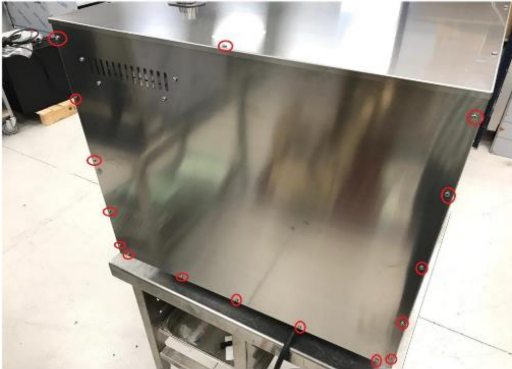
Figure 4. Removing the rear panel
