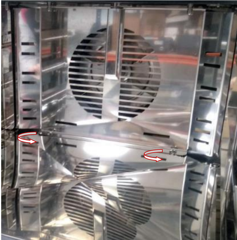
Figure 11. Removing the protective plate (screw models)
