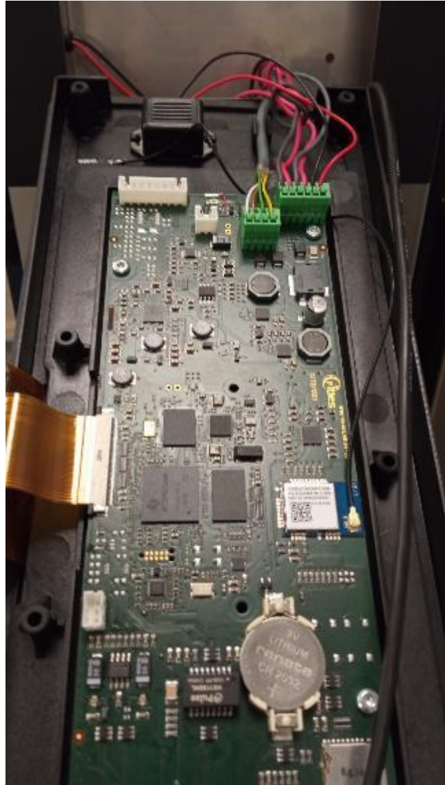
Figure 53. Connector release. (iCOOK, iBAKE) (See wiring diagram Figure 74)
