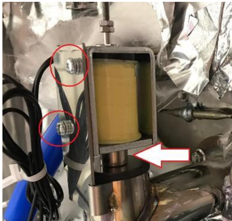
Figure 67. Disassembly of the solenoid
