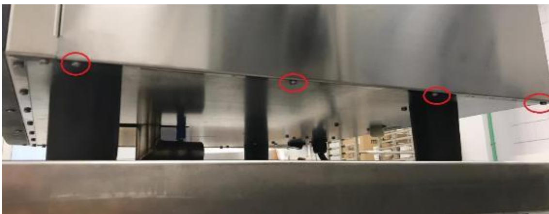
Figure 7. Lower screws on the side
