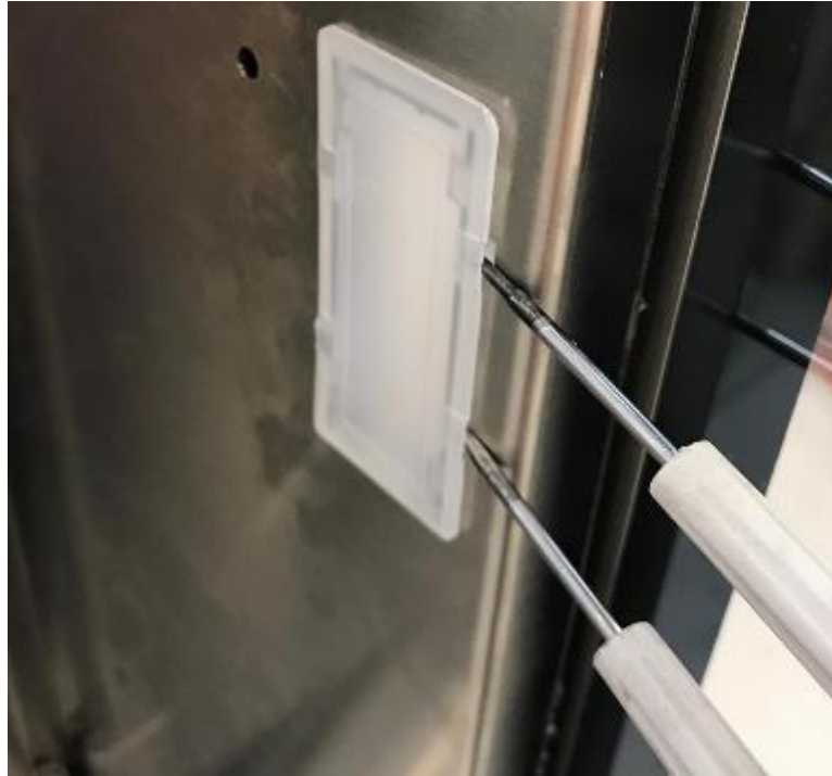
Figure 43. Replacement LED light. (COOK and BAKE)
