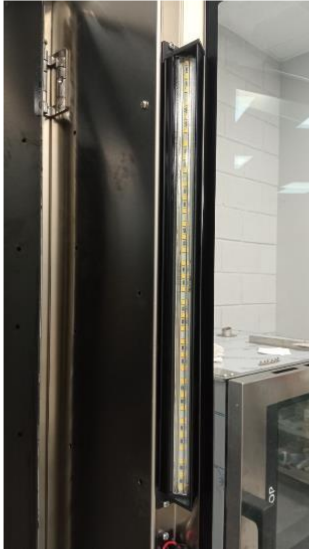
Figure 44. LED light replacement. (iCOOK and iBAKE)
