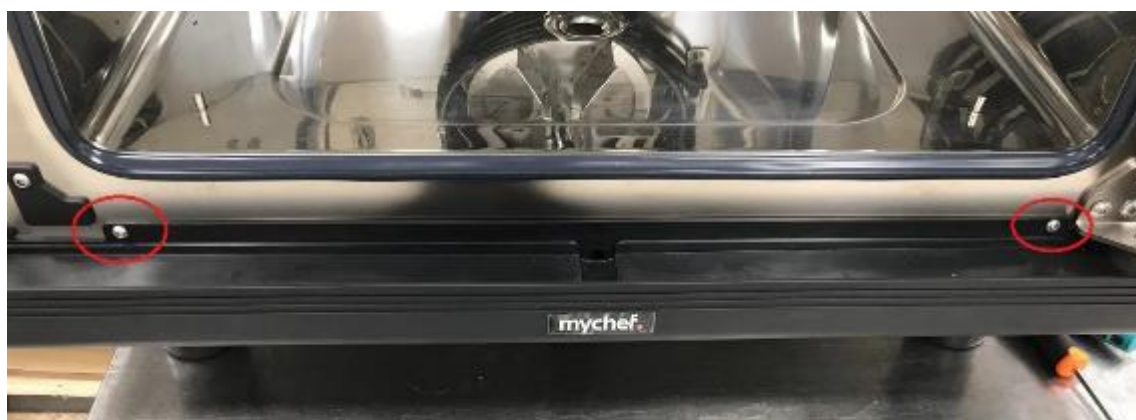
Figure 71. Upper drip tray screws
