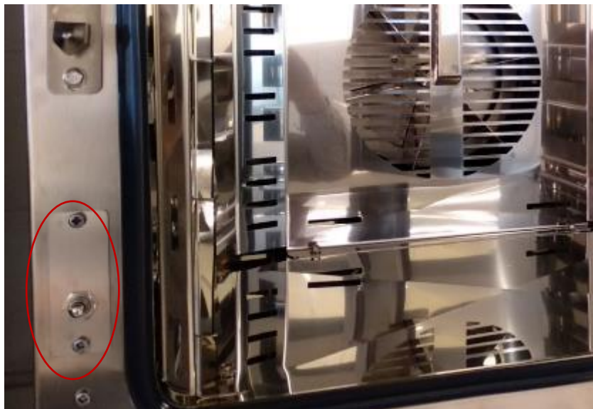
Figure 23. Door sensor (SNACK and BAKERSHOP)
