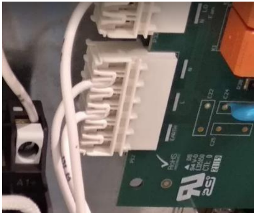
Figure 15. Checking input voltages (single-phase models)
