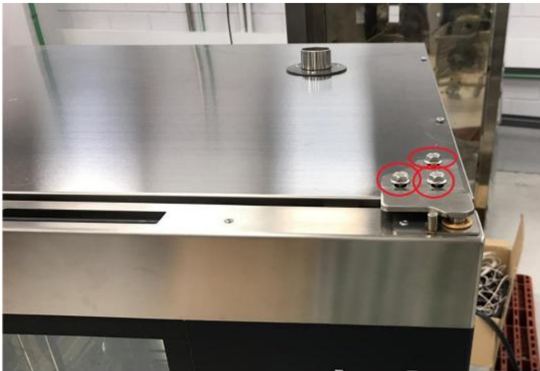
Figure 1. Removing the door (side-opening models)
