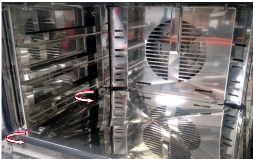
Figure 9. Removing the tray supports (screw models)
