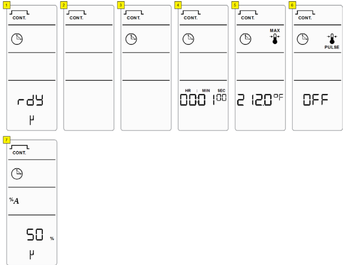
Figure 6.13 Temperature Limit - Continuous Sonics (Time) Mode
