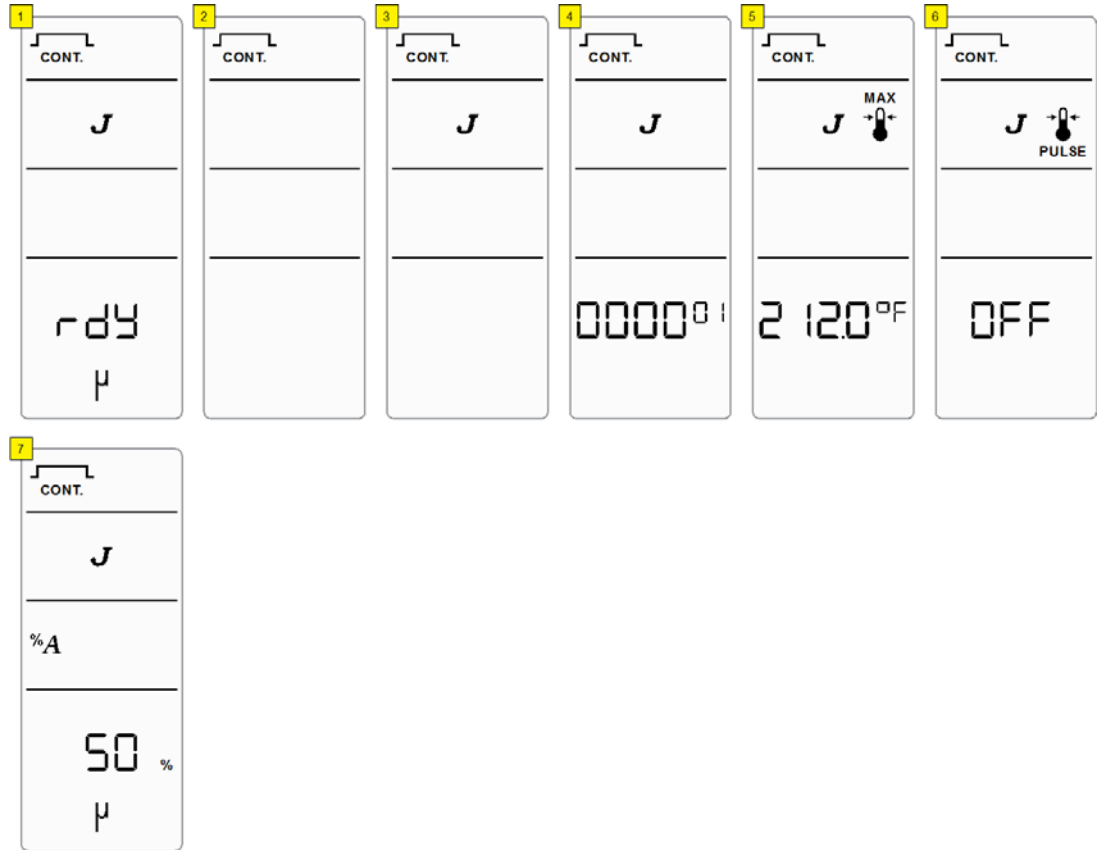
Figure 6.14 Temperature Limit - Continuous Sonics (Energy) Mode
