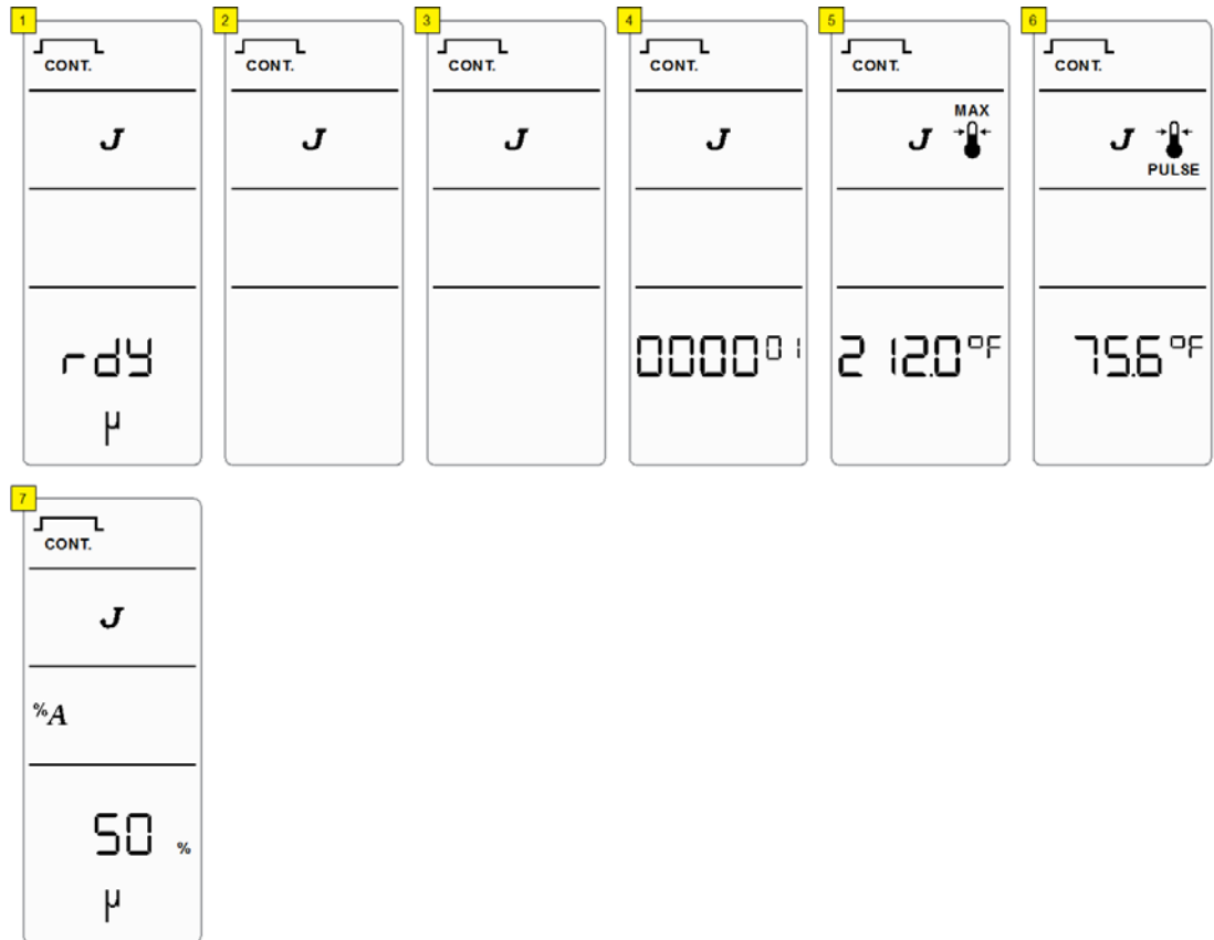
Figure 6.18 Pulse Temperature - Continuous Sonics (Energy) Mode
