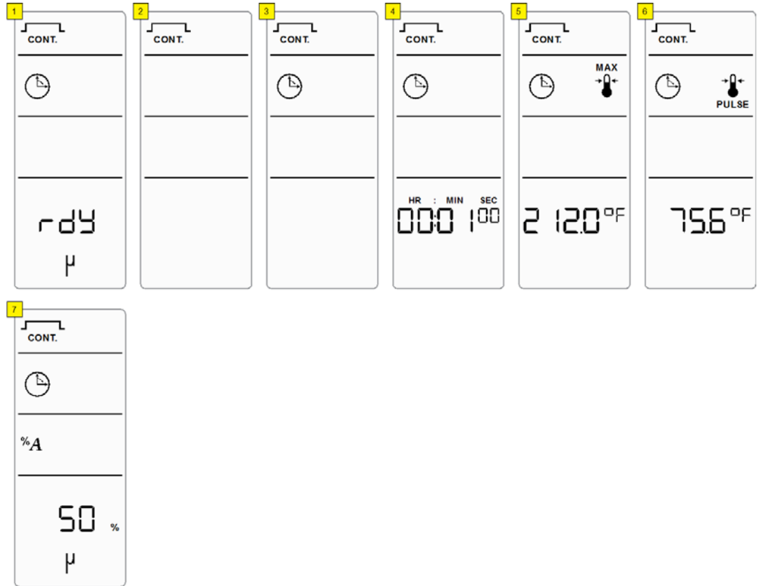
Figure 6.17 Pulse Temperature - Continuous Sonics (Time) Mode
