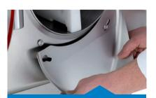
The extraction chute is removable to facilitate the removal of all gelato, cream, or chocolate residue, for complete cleaning. The cylinder and front panel are a single piece for maximum cleanliness and hygiene. This design also eliminates all gaps behind the paneling, where condensation and ice could work to shorten the life of the machine.
