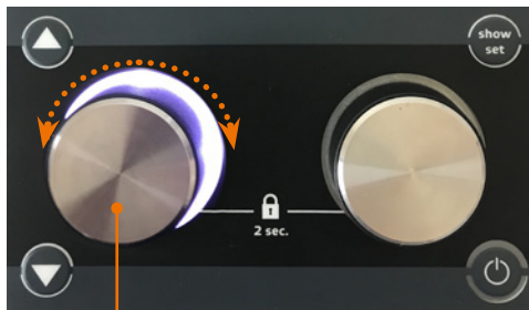
Rotation knob: Rotation switched on
