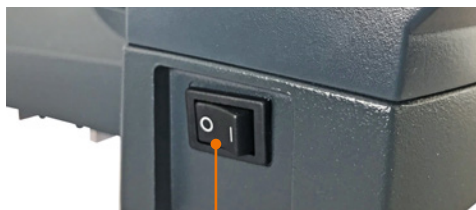
ON/OFF switch: OFF
